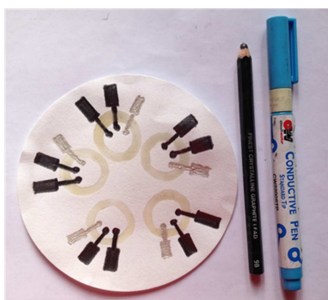
Figure 1. Five electrochemical paper-based devices developed on a filter paper. The silver conductive ink pen and 5HB pencil were used for the development of auxiliary and reference electrodes respectively. The working electrode is modified with alcohol oxidase enzyme.
