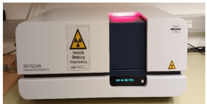
Figure 2 Table-top \mu CT scanner (SkyScan 1275, Bruker, Kontich, Belgium), equipped with a 100 kV microfocus X-ray source
